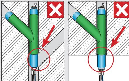
**NOTE!** Parts of the packer cover that is not covered by the feed branch pipe, must not be pressurized (installed) without being protected if it is in the open air, outside a pipe or there is another connection in the pipe to close the installation. Protect the exposed part of the packer cover with a piece of calibration hose, pipe or equivalent.
