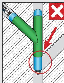
**NOTE!** Parts of the packer cover that is not covered by the feed branch pipe, must not be pressurized (installed) without being protected if it is in the open air, outside a pipe or there is another connection in the pipe to close the installation. Protect the exposed part of the packer cover with a piece of calibration hose, pipe or equivalent.
