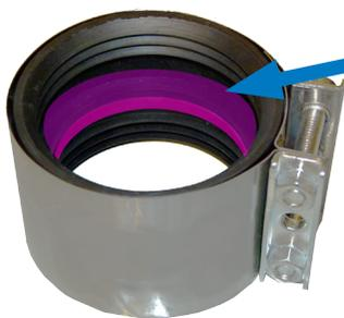
*Sealant is to be applied with a minimum 8mm filling up from the bigger ring in the rubber sealing.*
